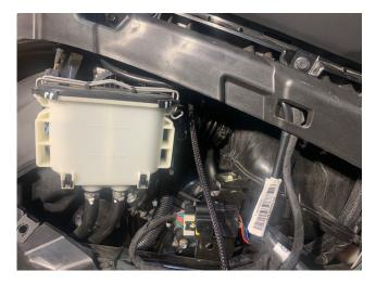
9.- The kit comes with the accessory power wire Y-Adapter that plugs into the Factory Accessory wire as shown below. Plug the supplied accessory wire into the factory plug as shown below. Then plug the docking station wire into the end of the Y-Adapter.
