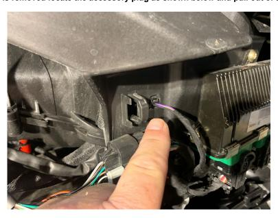
8.-Route the power wire from the docking down through the back of the steering area down through this area shown below.
