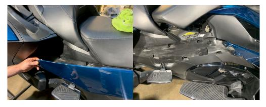
5.-Raise the seat to allow easier access to the docking station wiring. Next remove the upper blue panel shown below. Remove the 3 Torx screws shown. Then remove the 3 push pins under the front trunk.
