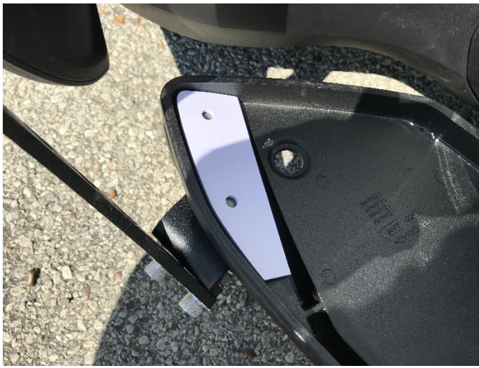
Left side install using drill template on Floor Board
