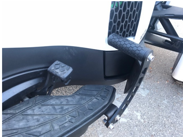
Right Side RT Road Peg Assembled on Floor Board
