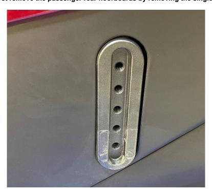
2.- Next as the photo above shows the left side of the RT take the left extender bracket and two of the black socket head bolts and washers supplied and install the bracket as shown below. You can adjust the bracket like the floorboard up or down. Once decided on the vertical position use
