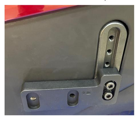
3.- Next take the existing floorboard and mounting bolt and locate it in the bracket. The extender bracket allows a 2" or 4" forward extended position from the factory original position. This allows the passenger to stretch their legs for a more comfortable ride. Test the positions to see what best fits you as a rider. Secure this existing OEM bolt with Blue Loctite. Do the same for the opposite side and your extenders are now installed.
