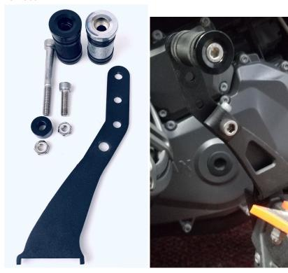
1.- First remove the existing factory shifter peg but loosening the socket head bolt that clamps the shifter peg to the factory arm. Once loosened remove that bolt to allow the factory shifter peg to be removed. It may take some wiggling to remove it.
