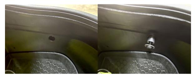
3.-Locate the bolt washer and spacer. Take the washer, place it on the bolt then add the spacer. Place through the hole as shown above then apple the flag holder to the outer trunk side once the paper template is removed.
