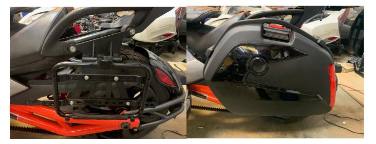
6.- Run the wires to the trunk and saddle bag for each side. Each side wiring harness does not matter which cable plugs into the ldle bag or the trunk. Be sure to wire tie the trunk wires as shown to existing wiring and all excess wiring to be wire tied up and placed next to the factory plugs, out of the way. Do the same for the other side.
