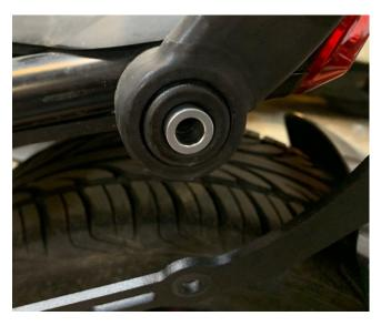
4.- Install the aluminum spacers as shown above in each location.
