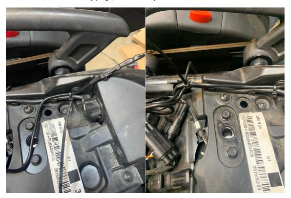
7.- Now check all wiring to assure that the brake, blinker and driving lights are working. If so, install the rear passenger seat and lock the rear trunk in place. Make sure, again the left & right taillight wires for the trunk are plugged in and working.
