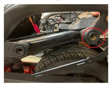
3.- When adding the new rear trunk rack assembly, it is best to have another person to help hold the mount in place while adding the spacers and bolts below. Start with the rear bolts Circled in Red above both sides first. Do one bolt each side at a time.
