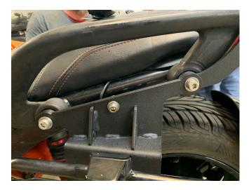
5.-Install the rear mount first then add the saddle bag brackets on top of the rear trunk mount as shown above.
