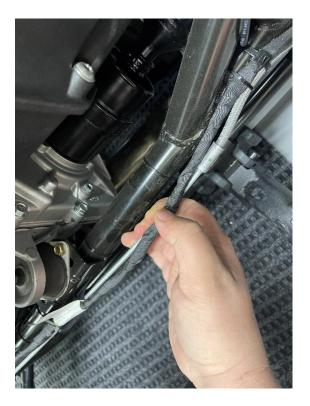
10. Gently pull back on the wiring and brake line to make sure there will be room to slide your frame mount bracket.
