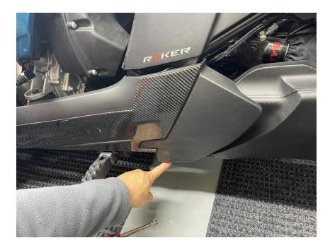
5. Locate the final push pin on the bottom of the side fairing in the rear to remove it.
