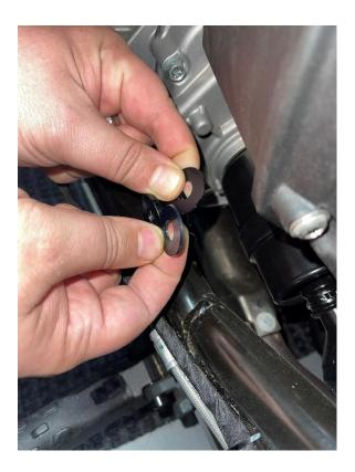
15. The nylon washers will go inside the vertical upright brackets of the frame mount.
