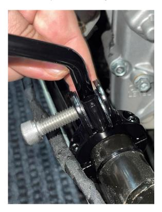
16. Place the vertical shaft in the middle of the two nylon washers and push the bolt through.
