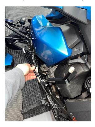
21. Hold the horizontal shaft to where the front ball joint hole lines up with hole on the outside edge of the shift lever. Make sure the factory shift lever is in the forward position.
