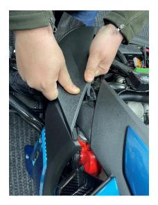
1. With the front hood removed pull down and towards the front of the bike on the front nose fascia to slide it off.
