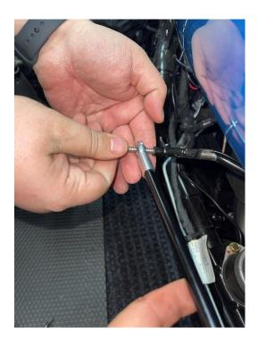
22. Insert the new longer torx 30 bolt and tighten all the way.
