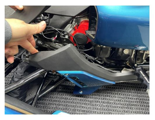
3. Pull outward on the side fairing releasing the push connector.
