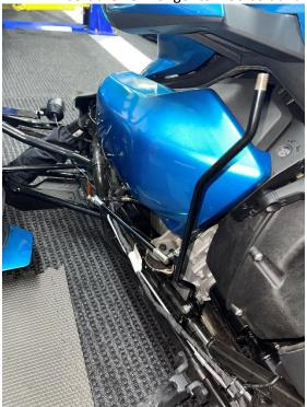
23. Carefully shift forward and reverse on your shift lever. Once in the forward position again your bracket should be sitting in the optimal position for functionality.
