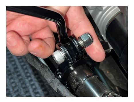
17. Attach the locking nut to the back and tighten until it is somewhat snug. Do not fully tighten yet.
