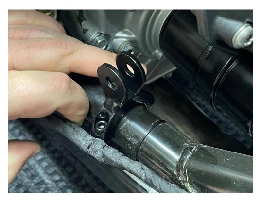
12. Lightly pull back the brake line as well as the wiring to affix the frame mount brackets.
