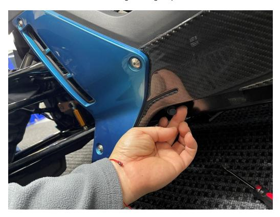
4. Locate the second push pin on the on side of the fairing towards the front and remove it.
