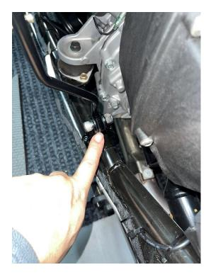
24. Come back through making sure all bolts are tight including the frame brackets which were loose up to this point.
